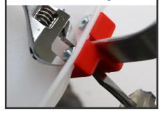
9. Push the sieve screen into place, being careful to push on the rubber outsides only.
