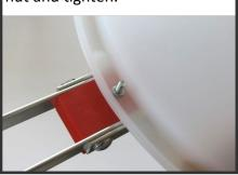
8. Insert short bolts through front frame clamps and bowl holes. Add nuts and tighten.
